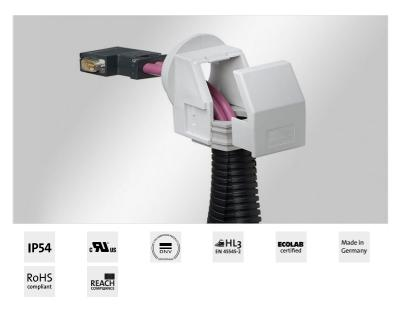
The split KVT-W90 cable glands are used to insert and seal pre-terminated cables at a 90° angle. But also electric, pneumatic or hydraulic lines without terminals or connectors as well as corrugated conduits can be easily routed (e.g. into control panels, enclosures or machinery) and sealed with IP54.
